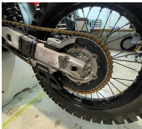
Touchless measurement System mounted on the rear wheel
